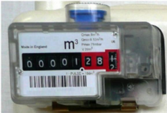
Metric meter registering in cubic metres (m<sup>3</sup>)
